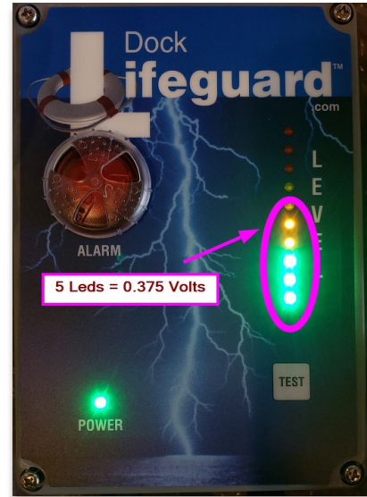
Three Switches in Closed Position, each LED = 0.12 Volts
