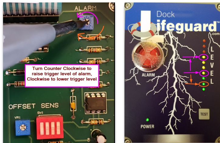
Adjusting Alarm Trigger Level
