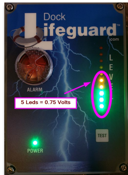
Two Switches in Closed Position, each LED = 0.16 Volts
