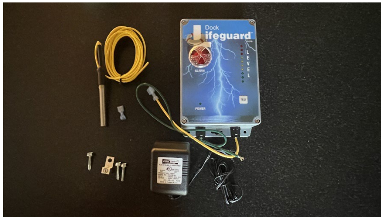
Figure 1, Dock Lifeguard Shock Warning System
