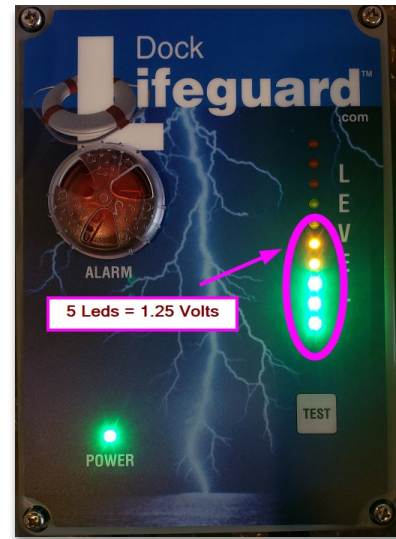
One Switch in Closed Position, each LED = 0.25 Volts
