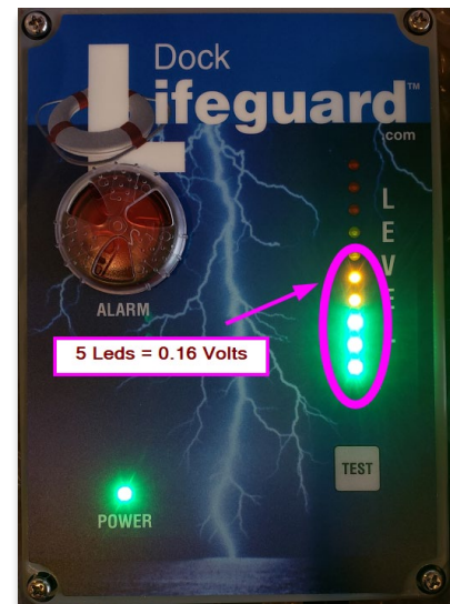
Four Switches in Closed Position, each LED = 0.08 Volts
