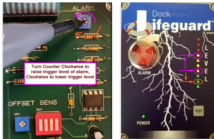
Adjusting Alarm Trigger Level
