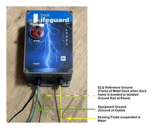
Note: If Metal Dock Frame is bonded to Equipment Ground of Outlet. The Green Wire and Green/Yellow wire can be tied together and attached to dock frame or the ground of outlet.
