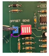
Sensitivity Settings: Internal dip switches allow for increasing the sensitivity level of the unit. Increasing sensitivity increases range of detection. Factory Defaults is one switch up (0.25Volts/LED) 0 = 0.5 Volts, 1 = 0.25 Volts, 2 = 0.16 Volts, 3 = 0.12Volts, 4 = 0.08 Volts
