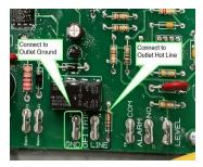
• **GFCI Trip**: By connecting a wire from the GFCI GND Tab to the Ground of an outlet, and wire from the LINE Tab to the Hot Wire of the outlet when the alarm sounds for 5 seconds, a pulse is issued to trip the GFCI breaker that is associated with that outlet. Test the GFCI tripping by pressing and holding the TEST button for 5 seconds. Warning: Wires should be in conduit.
